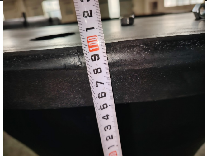
The GCO1000H rubber fender dimension checking
