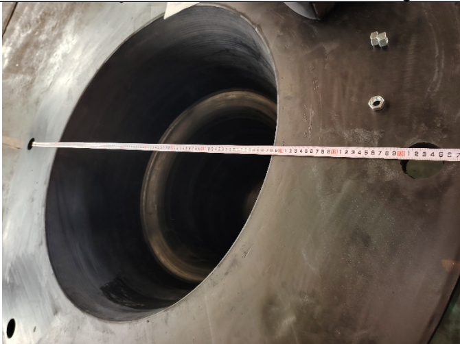
The GCO1000H rubber fender dimension checking
