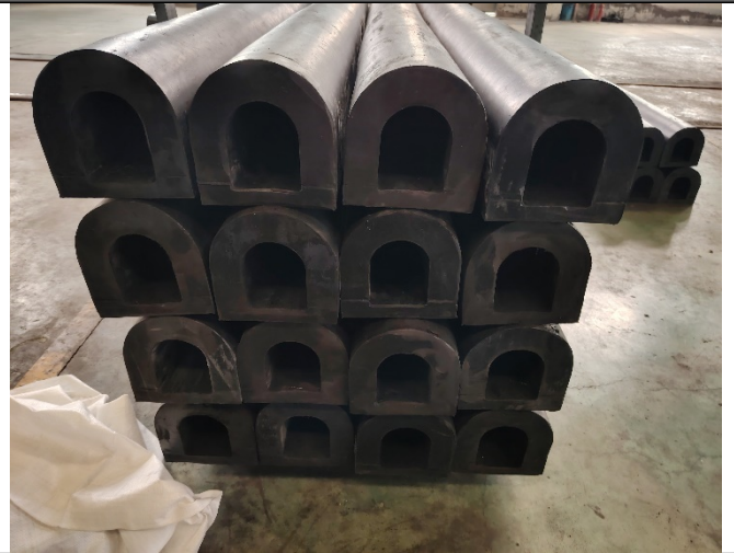
The GD250-2900 rubber fender visual and quantity checked
