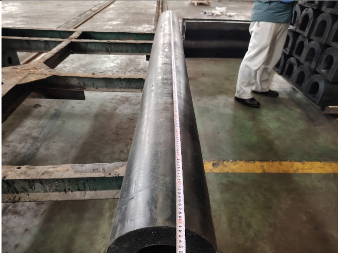
The GD250-2900 rubber fender dimension checked
