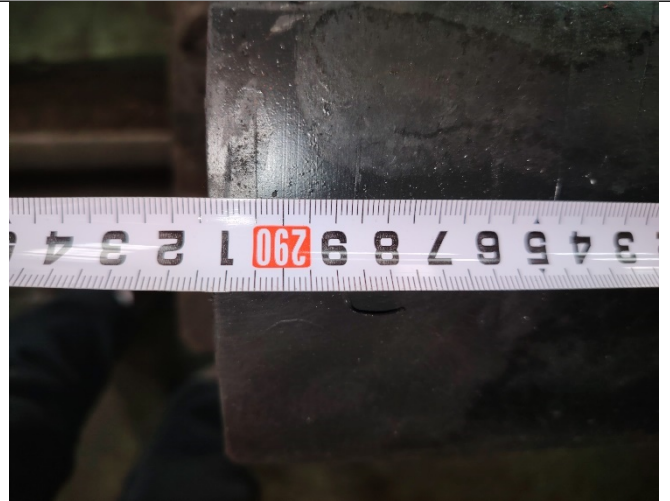
The GD250-2900 rubber fender dimension checked
