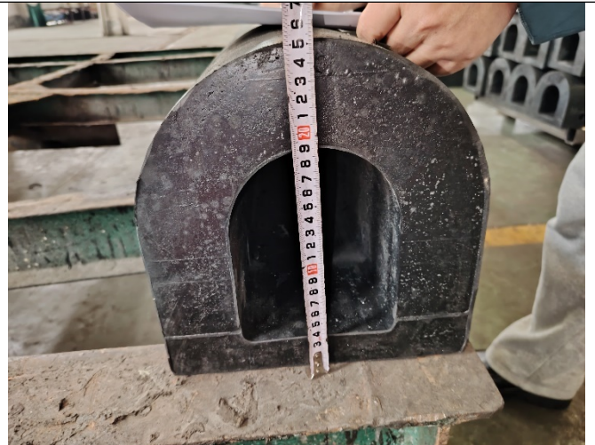
The GD250-2900 rubber fender dimension checked
