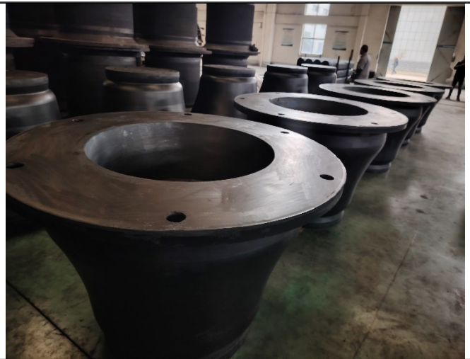
The GCO1000H rubber fender visual and quantity checked
