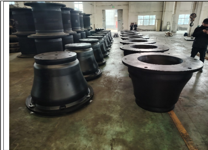
The GCO1000H rubber fender visual and quantity checked
