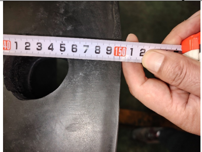
The GCO1000H rubber fender dimension checking
