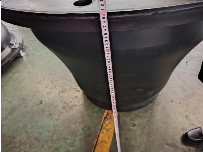
The GCO1000H rubber fender dimension checking
