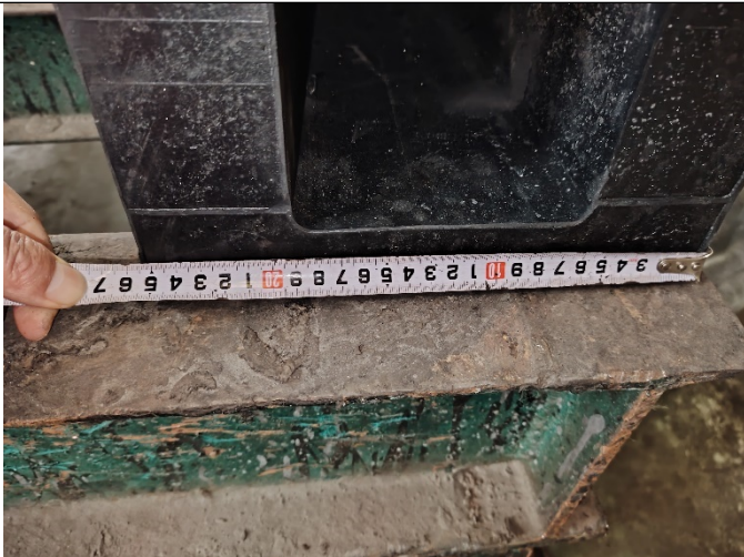
The GD250-2900 rubber fender dimension checked
